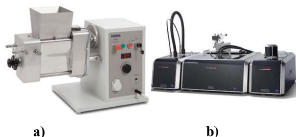
Figure 1. Wet Granulator with oscillating rotor - a) and ANALYSETTE 22 NanoTec plus - b)
