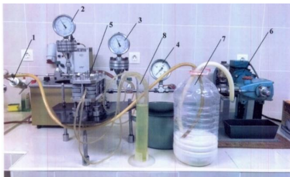
Figure 1. Scheme of laboratory equipment with a replaceable plate and frame membrane module 1 – valve; 2, 3, 4 – manometers; 5 – replaceable plate and frame membrane module; 6 – pump; 7 – tank for initial solution; 8 – cylinder for permeate
